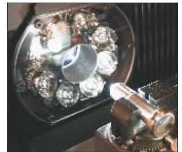
TruLight oblique ring light is standard on CC-16L.
