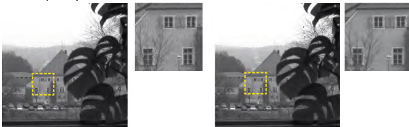
Figure 27: The left image shows an uncorrected image, obtained with tap A readout, while the right image shows the result image after an asymmetry correction, where the same image was read out from tap B as well, and both images have been averaged. The small images represent an extract of the area, which is denoted by the yellow square.
