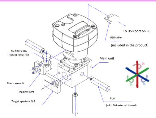
%1 Applicable optical filter size:  $\phi$  9 mm to  $\phi$  10 mm, thickness 3 mm to 5 mm (Please prepare by customer if necessary)
