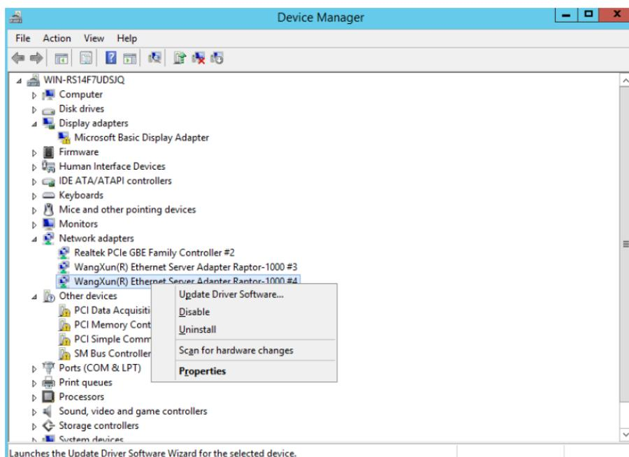
在提示框中勾选删除该设备的驱动程序 Delete the driver software for this device, 单击 OK。
