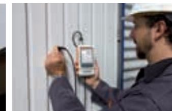
Measurement of a paint coating on steel
