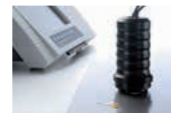
Hand probe with beta emitter
