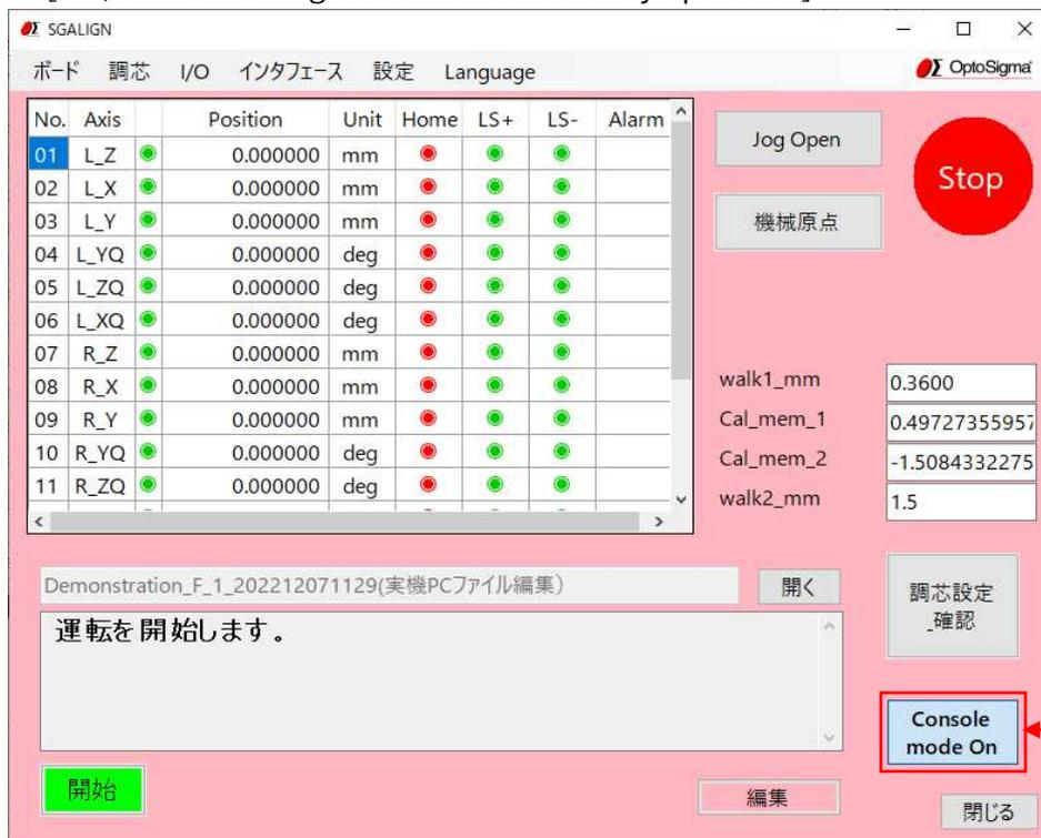
ON/OFF switching button for console key operation
